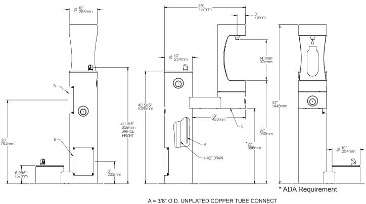
A = 3% O.D. UNPLATED COPPER TOBE CON SHUT OFF VALVE BY OTHERS B = ACCESS PANEL (8" x 10")
