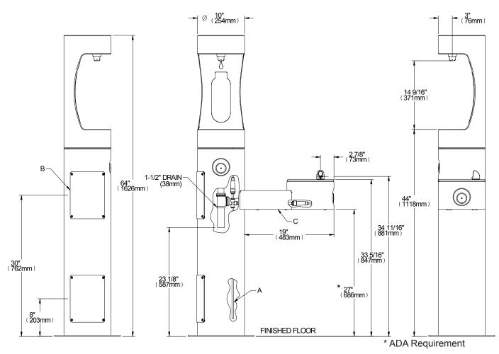
A = 3/8" O.D. UNPLATED COPPER TUBE CONNECT SHUT OFF VALVE BY OTHERS
